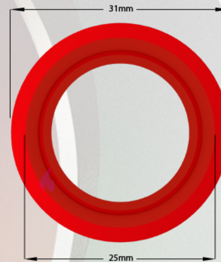
Jointing Socket Front Elevation
